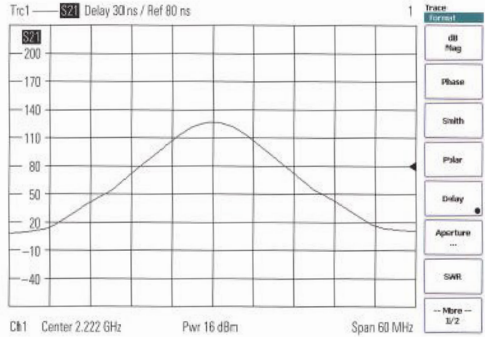
Fig.4.5.6 Group delay for Fig. 4.5.3 with aperture stepwidth 100 (too large).
